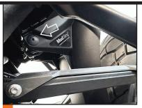
INSERT a New plastic screw in the upper LEFT side hole of the MudSling. Push and Screw it in until firmly seated.
