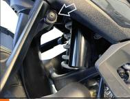
INSERT a New plastic screw in the upper RIGHT side hole of the MudSling. Push and Screw it in until firmly seated.
