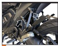
OPTIONAL: To provide sufficient working room, temporarily remove the Left side passenger footpeg using a T40 Torx socket wrench.
