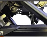
Remove the plastic screws holding both Left and Right sides of the Center Cover. Do Not remove cover.
