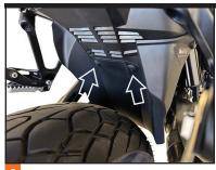
Position the MudSling over the BMW cover to align with the 2 central holes. Push-in 2 New Screws and Screw in until firmly seated.
